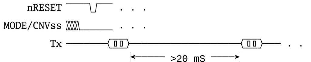
After sending the last byte, wait 2mS and then read any data that might have been sent back to the host. Sometimes there's a glitch at reset that looks like a byte, and some chips transmit a byte at the end of synchronization. By reading these optional bytes and clearing your receive buffer, you ensure you're in sync with the bootloader.
