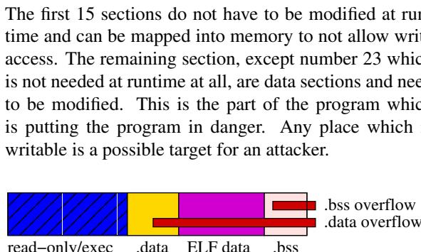
This graphic shows the different parts of the ELF file. The hatching indicates the memory is write-protected. The red bars indicate which areas a potential buffer overrun in the `.data` and `.bss` section respectively can easily affect.
