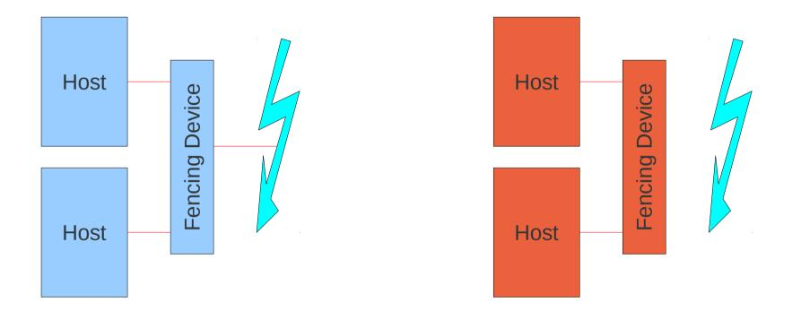
• One power cord = Single Point of Failure
