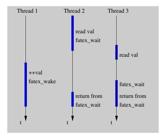
This diagram represents the execution of a program with three threads. Each thread's execution is represented by a vertical line, progressing with time downward. The blue parts are those at which the thread actually has a CPU. If two or more blue lines overlap vertically the threads are executed concurrently.
